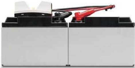
UPS-BAT/VRLA-WTR... (Valve Regulated Lead Acid/ Wide Temperature Range) – Tempos de buffer máximos com temperaturas extremas – Tecnologia AGM (Absorbent Glass Mat) de chumbo puro
